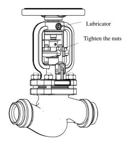
Leakage on the gland packing means that bellow was damaged. Upper part of the valve should be replaced immediately
