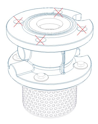
It is not allowed to fit lifting devices to connecting holes.
