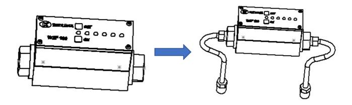
6.3. Attach the indicator with the tubes to the filter with the screwed reducers. Remember that the direction of flow on the indicator and filter should be the same.
